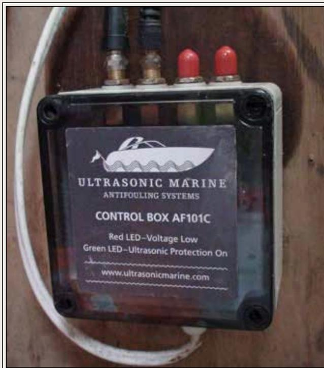
Aboard my 34-footer, *Gypsy Wind*, I installed a pair of transducers (left). Where you position them is critical to the effectiveness of the system. When installing, wriggle the unit into the epoxy to eliminate any air bubbles. The heart of the Ultrasonic system is the control box (right). Wiring is simple, with the power line clipped into the bottom of the unit, and the transducers into the top.
