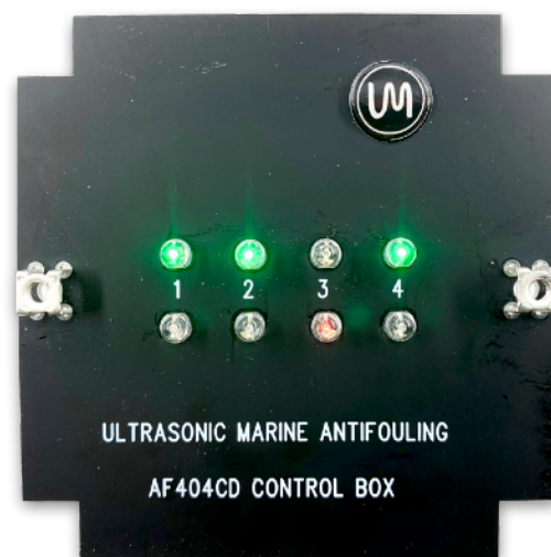
Channel 3 in Alarm
